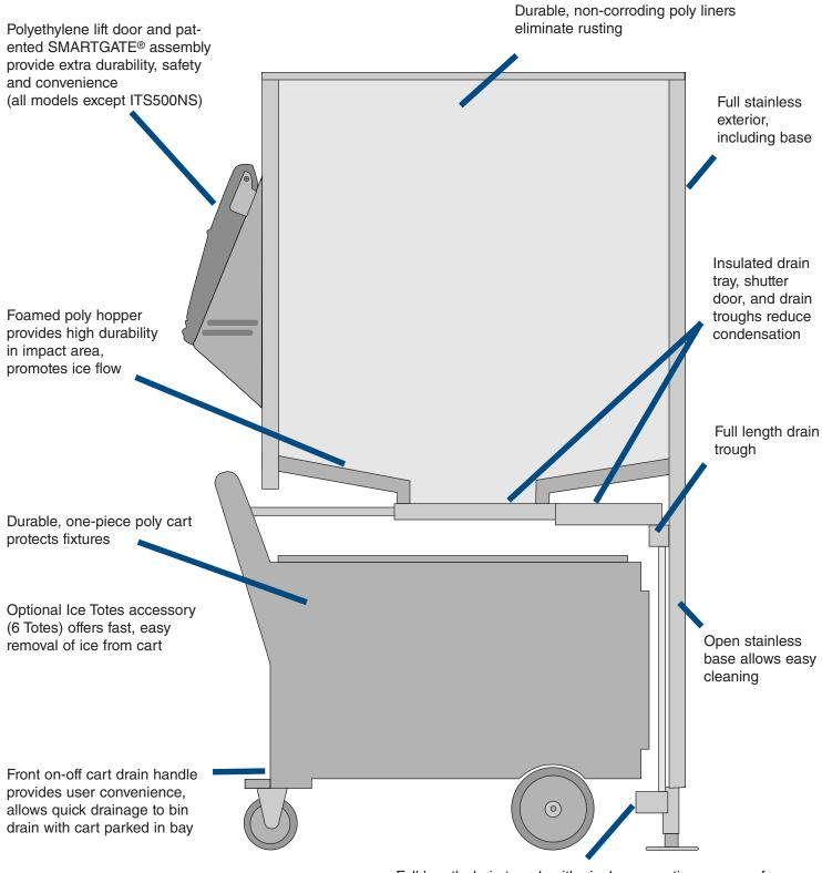
Full length drain trough with single connection reverses for best access to floor drains
