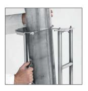
The strainer cylinder and screw conveyor are easily accessible and removable.
