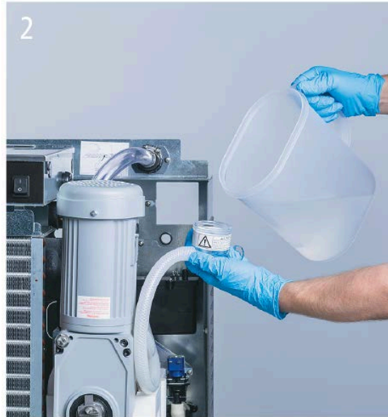
2 – Fill cleaning cup with SafeCLEAN Plus™ cleaning solution until HI WATER light comes on. The ice machine does the rest!
