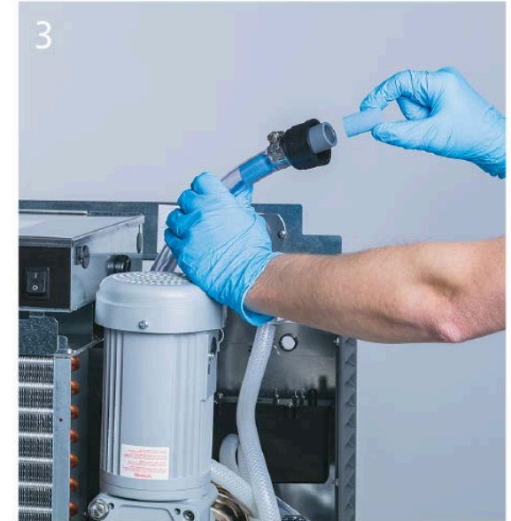
3 – Insert a dry SaniSponge™ followed by a sponge soaked in SafeCLEAN Plus cleaning solution. As ice is harvested, it will push the sponges through the ice transport tube to sanitize it. Catch and discard the sponges and a small amount of ice.
